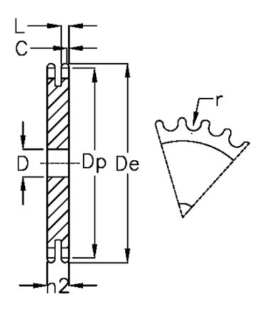
C = 2 D = 25 De = 331.5 Dp = 323.53 For chain size =  $5/8 \times 3/8$ For chain type = 10 B-2 h2 = 25.5
